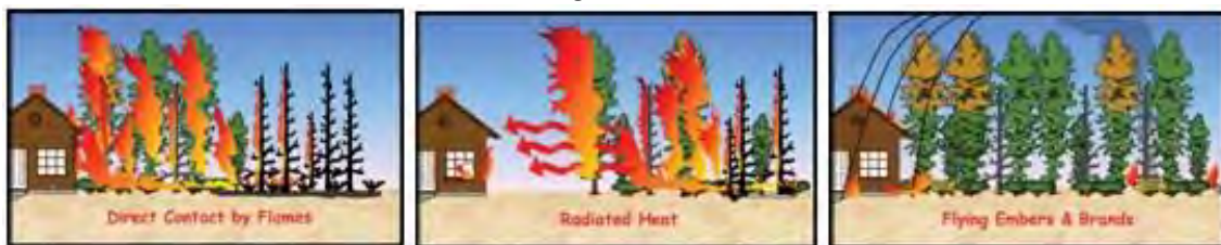
Three Forms of Structure Ignition (from www.firewise.com )
